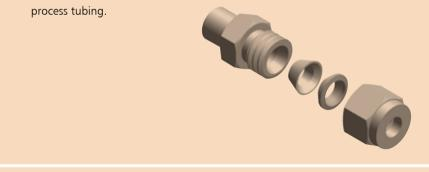
• VCR® adaptors are used to connect a male or female VCR component to an existing flange system. VCR's seal by the compression of a gasket (usually copper) between two highly polished beads on the surfaces of the VCR connectors.
